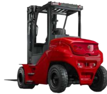
ELECTRIC COUNTERBALANCE FORKLIFT From 2.5 - 10.5T capacity
